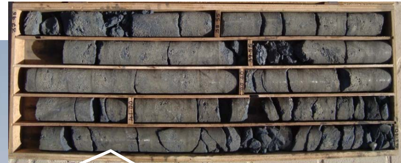
Core hole DEDC002 6m massive sulphides intersected at 37-43m
