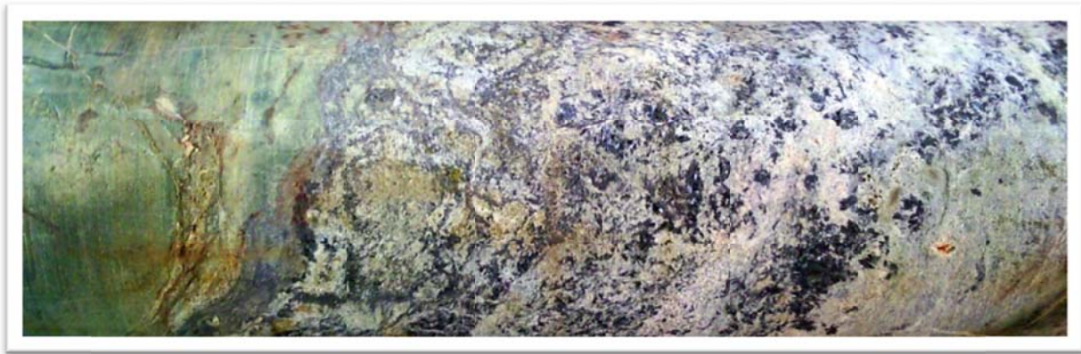
Core from the Khnaiguiyah Project showing intersection containing Sphalerite ((Zn, Fe) S) mineralisation. (Sphalerite is a zinc/iron sulphide and the primary ore of zinc metal.)
