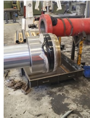
Image 2: Rectification of damaged cylinder
