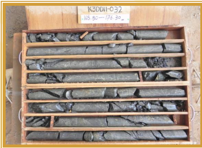
High grade zinc and copper intersections in Drill Hole K3DD11_032 at Zone 3
