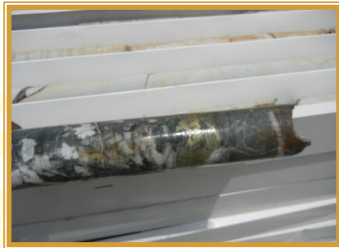
Drill Hole core from Zone 3 showing chalcopyrite veins
